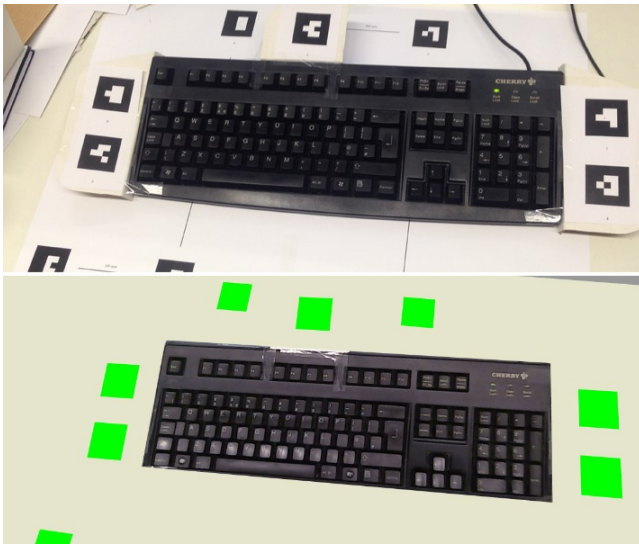
Figure 2: The upper image is showing a keyboard on a common office desktop that is tracked by a webcam and some markers to be prototypically placed on a virtual desk in the virtual environment (lower image). Thus the user can use her keyboard for text input in the IVE.
