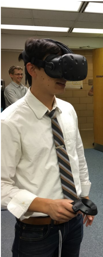
Figure 4: An expert user experiencing our prototype system. This illustrates two main components of the HTC vive hardware: the tethered HMD and the wireless hand controller (only one pictured).
