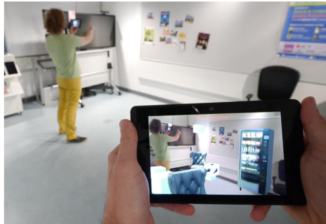
Figure 1. Collaborative Mixed Reality (MR) experience with MR tablets [18]. Two collaborators can explore digital information which is integrated in their physical environment and represented as virtual objects.
