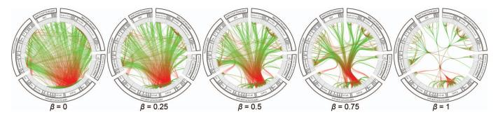
Fig. 14. Using the bundling strength  $\beta$  to provide a trade-off between low-level and high-level views of the adjacency relations. The value of  $\beta$  increases from left-to-right; low values mainly provide low-level, node-to-node connectivity information, whereas high values provide high-level information as well by implicit visualization of adjacency edges between parent nodes that are the result of explicit adjacency edges between their respective child nodes.
