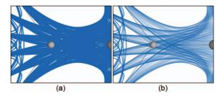
Fig. 10. Alpha blending helps to distinguish individual curves or subbundles within a bundle. (a) Alpha blending disabled; (b) alpha blending enabled.
