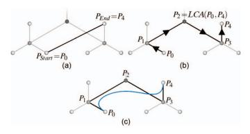
Fig. 3. Bundling adjacency edges by using the available hierarchy. (a) Straight line connection between  $P_0$  and  $P_4$ ; (b) path along the hierarchy between  $P_0$  and  $P_4$ ; (c) spline curve depicting the connection between  $P_0$  and  $P_4$  by using the path from (b) as the control polygon.
