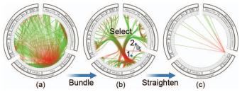
Fig. 16. Bundle-based interaction. (a) A user starts with a low-level view; (b) the bundling strength is increased and areas of interest emerge as bundles, which can be selected by dragging a line through them; (c) only selected curves remain visible and the user returns to an uncluttered low-level view to further inspect individual curves.
