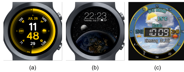
Figure 5.1: (a) A donut chart that uses the circumference of the round watch face; (b)(c) the graph for moon phase and weather that fill the whole watch face. Taken from Facer [11] and Watchmaker [29].
